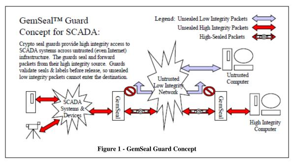
the canonical representation of the source network sensitivity level are included in the CBC computation of the seal. The seal is the final encryption block of the CBC-mode encryption of the packet source-network sensitivity label (canonical representation) and contents of the packet, using a packet-specific initialization vector (IV) and the configured sensitivity level secret key.
