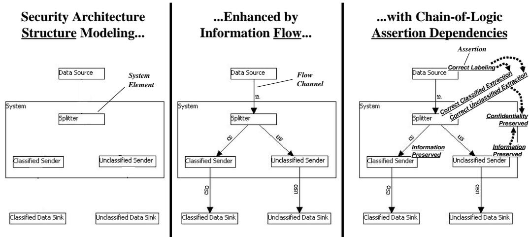
Figure 2. BFM Construction Phases
